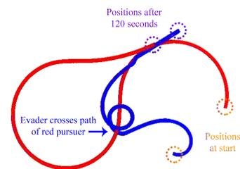
Figure 6: Pursuit-evasion by a fast pursuer with a low turning velocity (a Homicidal Chauffeur).
