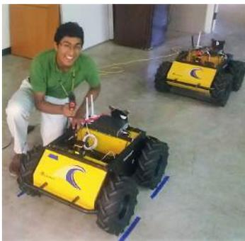
Figure 4: The Clearpath Husky A200 robot platform.
