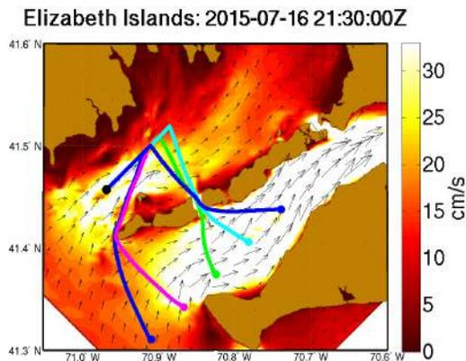
Figure 3: Underwater robot path plans in dynamic ocean currents off of the Elizabeth Islands of Massachusetts for intercepting a moving ship.
